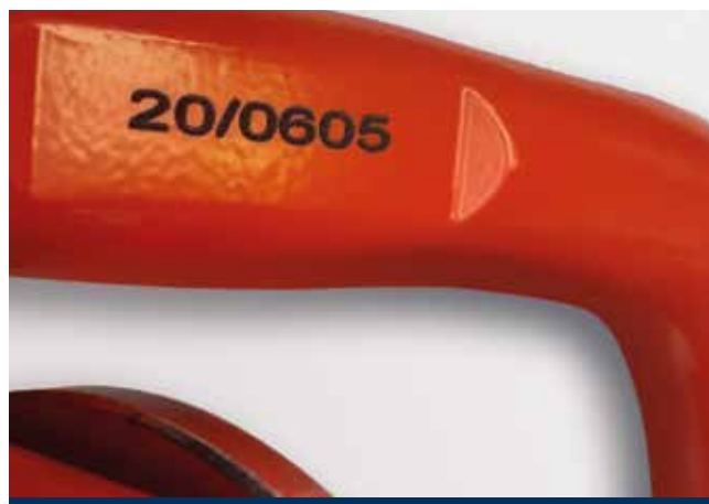
Laser engraved marking of the serial number
